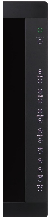
LMD-2451MT sheet-type switches on the front bezel
